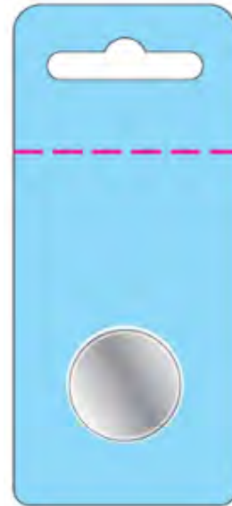
Perforation in adhesive part
