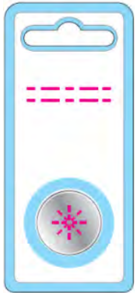
Perforation for air inlet and other perforation
